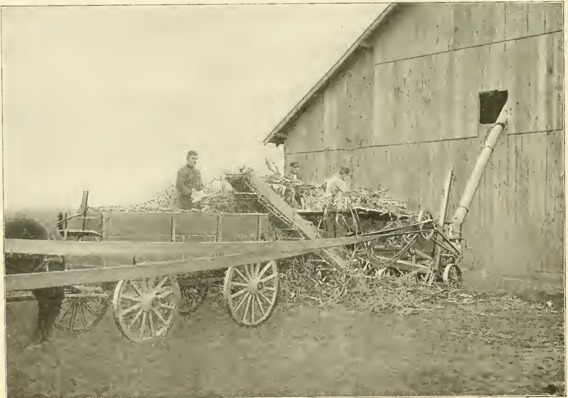
The Deering 6-roll husker and shredder is an ideal machine for its purpose
