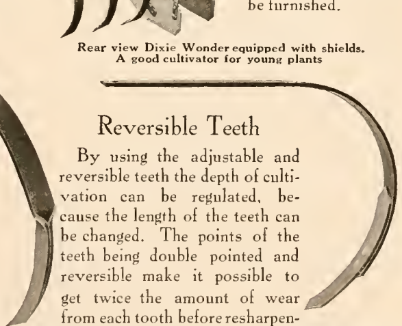
Adjustable and reversible tooth, furnished on special order
